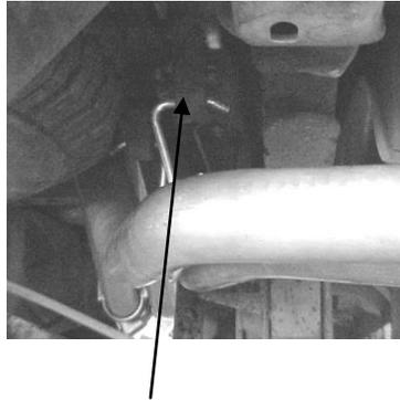
NEXT INSTALL PASSENGER OVERAXLE # C. INSERT WELDED HANGER INTO RUBBER GROMMET. DO NOT TIGHTEN. ATTACH TAILPIPES TO THE MUFFLER USING CLAMPS # F. USE BOLT KIT # I TO ATTACH BOTH OVERAXLE PIPES TOGETHER.
