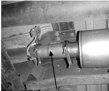
INSTALL HEADPIPE # A USING CLAMP # F AND ATTACH TO THE STOCK EXTENSION PIPE. INSTALL THE MUFFLER USING CLAMP # G. USE JACKSTANDS TO SUPPORT THE MUFFLER. DO NOT TIGHTEN.
