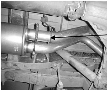
INSTALL REAR TAILPIPE HANGER # H ON THE DRIVERSIDE INTO THE RUBBER GROMMET. SLIDE THE DRIVERSIDE OVERAXLE TAILPIPE # D THRU THE HANGER THEN INSERT WELDED HANGER INTO RUBBER GROMMET. ATTACH WITH CLAMP # F TO MUFFLER.
