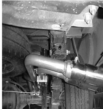
ROLL TAILPIPES UNTIL YOU HAVE IT AT THE CORRECT ANGLE FOR YOUR VEHICLE. NOW FIRMLY TIGHTEN ALL BOLTS, CLAMPS, AND FLANGES.
