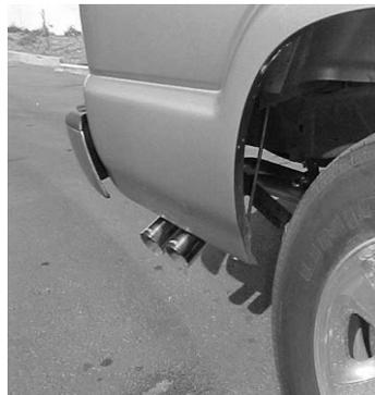
INSTALL STAINLESS STEEL TIPS. USE ANY ALUMINUM OR STAINLESS STEEL CLEANER TO POLISH TIPS.
