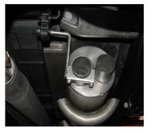
INSTALL MUFFLER #B ONTO HEADPIPE 1-1/2" TO 2". USE CLAMP #J TO SECURE THE MUFFLER TO THE HEADPIPE. DO NOT TIGHTEN. INSTALL REAR MUFFLER HANGER #F ONTO THE DRIVERSIDE MUFFLER OUTLET. INSERT WELDED HANGER INTO RUBBER GROMMET. DO NOT TIGHTEN.
