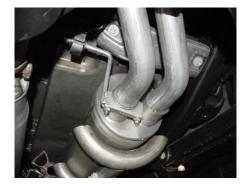
INSTALL PASSENGER SIDE TAILPIPE #D INTO MUFFLER 1-1/2 TO 2". INSERT WELDED HANGER INTO RUBBER GROMMET. USE CLAMP #I TO SECURE THE TAILPIPE TO THE MUFFLER. DO NOT TIGHTEN.
