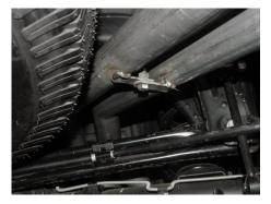
INSTALL DRIVERS SIDE TAILPIPE #C INTO THE MUFFLER 1-1/2" TO 2". USE BOLT KIT #H TO SECURE THE TAILPIPES TOGETHER. DO NOT TIGHTEN. DRIVER SIDE TAILPIPE WILL BE ON TOP OF PASSENGER SIDE TAB.
