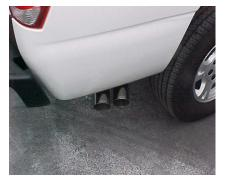
INSTALL THE STAINLESS TIPS. NOW GO BACK AND TIGHTEN ALL THE CLAMPS, NUTS AND BOLTS STARTING FROM THE FRONT AND WORKING BACK. TO CLEAN THE TIPS USE ANY STAINLESS CLEANER AND A SCOTCH BRITE PAD.
