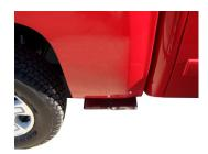
5. Install right and left stainless steel tips. Clamp down. When you have everything in place, firmly tighten all bolts and clamps down securely. Use stainless steel cleaner and a Scotch Brite pad weekly to prevent tip from discoloration. Inspect all fasteners after 25-50 miles of operation and retighten as necessary.
