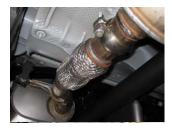
2. To remove stock exhaust, the Y-pipe. Make sure to leave all rubber grommets in the factory location. **You will reuse stock clamp.** For easier removal of exhaust, cut behind the muffler. Use WD-40 to remove hangers from grommets.
