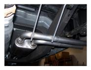
4. Rotate the muffler assembly until the outlets are level.
