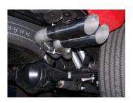
7. Use bolt kit #h to attach tailpipe tabs together.
