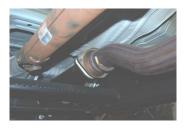
2. To remove your stock exhaust, unbolt the 2-bolt flange located in front of the muffler. Disengage the welded hangers from the rubber grommets. Use WD-40 to aid in this process. Do not remove or damage the rubber grommets as you will reuse them to mount your new system. Now, cut off tailpipe and remove exhaust. Do not throw away stock hardware.
