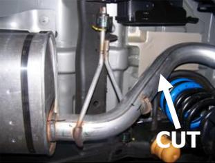
**2.** To remove the stock exhaust, Un clamp it from the clamp in front of the muffler. Do not disguard you will re-use clamp. Disengage the welded hangers using WD-40 from the OEM rubber grommets. Do not damage or remove the rubber grommets as you will reuse them to mount your new system. Now, cut off tailpipe before and after rear axle for removal.
