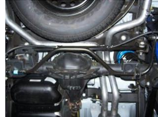
**7.** Install driver side tailpipe #C to the muffler 1 1/2"-2". Use clamp #G to secure tailpipe to muffler. DO NOT TIGHTEN. Insert welded hangers into rubber grommets.
