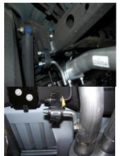
7. Install driver's side rear hanger #M onto side of frame as seen in picture. Secure bolt kit #O to frame. Use grommet #L and clamp hanger #N. This clamp also holds exit pipe to tailpipe.
