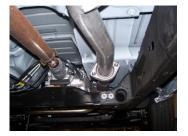
3. **2009/2010 Models Only** You will use part "N" to attach to the muffler re-using the factory clamp. Be sure that the tabs of the clamp are straight. If they are bent, it will not seal the connection.
