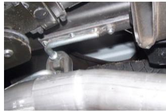
6. Install metal hanger #I into hole located in front of the rear leaf spring stock mount.
