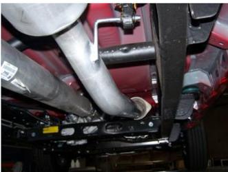
3. Install headpipe #A onto your existing stock front headpipe using stock hardware to secure pipes together. Do not tighten. Insert welded hangers into rubber grommets.
