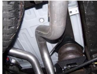
5. Slide the over axle tailpipe #C into the muffler 1.5-2". Use clamp #E to secure tailpipe to muffler. Do not tighten. Insert welded hangers into rubber grommets.
