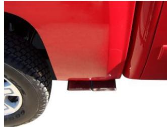
6. Install right and left stainless steel tips. Clamp down. When you have everything in place, firmly tighten all bolts and clamps down securely. Use stainless steel cleaner and a Scotch Brite pad weekly to prevent tip from discoloration. Inspect all fasteners after 25-50 miles of operation and re-tighten as necessary.
