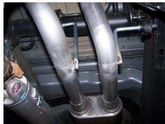
7. Using clamps #G secure both tailpipes to the outlets of the muffler. Rotate tailpipes to best fit your truck.
