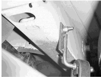
Install tailpipe hanger #J on the frame, then measure 9" from the rear; you will see a 1" round hole use this to mount your hanger. Use the bolt kit and rubber grommet provided in your kit.
