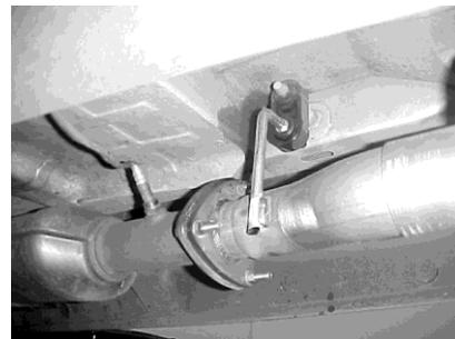
Install your head-pipe # A onto your existing stock flange, use your supplied hardware # M & gasket # N in the kit. Use a jack stand to support the converter. Insert the welded hanger into the rubber grommet.
