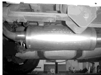
Install muffler #B onto head-pipe #A 1-1/2" to 2" with the louvers in the muffler facing towards the converter. Use a jack stand to support the muffler. Use Clamp #G to secure the muffler to the head-pipe. **Do Not Tighten at this Time!**
