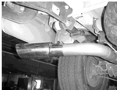
Next, install the exit pipes #E. Use clamps # I to secure them. Insert welded hangers.
