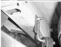
Install tailpipe hanger #J on the frame, then measure 9" from the rear; you will see a 1" round hole use this to mount your hanger. Use the bolt kit and rubber grommet provided in your kit, # K & L
