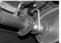
Lay out the exhaust on the floor so it looks like the drawing and compare the parts with the manual. To remove the stock exhaust, un-bolt it from the 3-bolt flange located in front of the muffler. NOTE: For an easy removal of the exhaust, cut the tailpipe off behind the muffler. Leave all rubber grommets in place. Use WD-40 to aid in removal.
