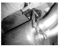
Install rear muffler hanger #H.
