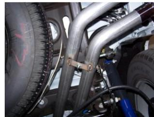
**8.** Install stainless steel tips #G. Clamp down. When you have everything in place, firmly tighten all bolts and clamps down securely. Use stainless steel cleaner and a Scotch Brite pad weekly to prevent tip from discoloration. Inspect all fasteners after 25-50 miles of operation and re-tighten as necessary
