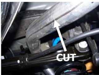
**3. 2009-10 Models Only** Measure 8" from the flange on your new headpipe #A and cut. Attach adapter pipe to new headpipe with the 3" clamp. You will re-use the factory band clamp.
