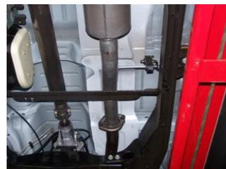
**4.** Install muffler #B onto head pipe #A 1½"-2". Muffler outlets will be positioned at the top. Use a jack stand to support the muffler. Use clamp #E to secure the muffler to the headpipe. DO NOT TIGHTEN.
