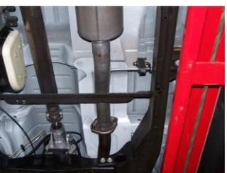
**5.** Remove spare tire to install tailpipes. Now install passenger side tailpipe #D into the muffler 1 1/2"-2". Use clamp #G to secure tailpipe to muffler. DO NOT TIGHTEN. Insert welded hangers into rubber grommets.
