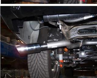
**9.** Install stainless steel tips #J. Clamp down. When you have everything in place, firmly tighten all bolts and clamps down securely. Use stainless steel cleaner and a Scotch Brite pad weekly to prevent tip from discoloration. Inspect all fasteners after 25-50 miles of operation and re-tighten as necessary.
