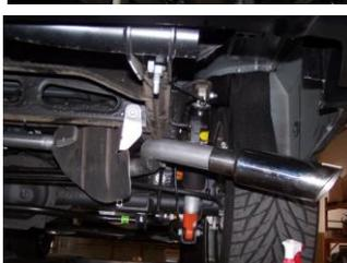
**4.** Install muffer #B onto head pipe 1 1/2"-2" with the louvers facing towards the converter. Use a jack stand to support the muffer. Muffer outlets will be positioned at the top. Use clamp #F to secure the muffer to the headpipe. DO NOT TIGHTEN.
