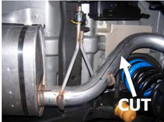
**2.** To remove the stock exhaust, unbolt it from the two bolt flange in front of the muffler. Do not disguard you will re-use bolts. Disengage the welded hangers using WD-40 from the OEM rubber grommets. Do not damage or remove the rubber grommets as you will reuse them to mount your new system. Now, cut off tailpipe before and after rear axle for removal.
