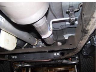
Bolt head pipe #A onto your existing stock front pipe re-using stock nuts/bolts. Insert welded hanger into rubber grommet. DO NOT TIGHTEN.
