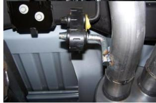
**8.** Install driver side tailpipe #C to the muffler 1 1/2"-2". Use clamp #H to secure tailpipe to muffler. DO NOT TIGHTEN. Insert welded hangers into rubber grommets.
