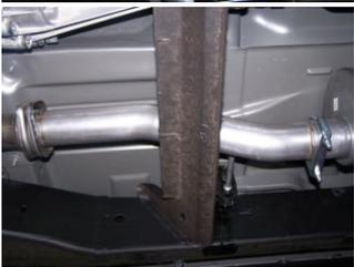
Bolt head pipe #A onto your existing stock front pipe re-using stock bolts. Use a jack stand to support the converter. Insert welded hanger into rubber grommet. DO NOT TIGHTEN.
