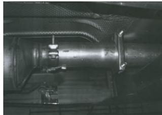
**4.** Install muffler #B onto head pipe #A 1 1/2"-2". Use a jack stand to support the muffler. Use clamp #G to secure the muffler to the headpipe. DO NOT TIGHTEN.
