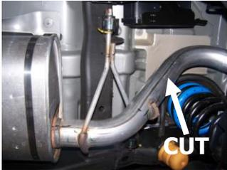
**2.** To remove the stock exhaust, remove it from the two bolt flange in front of the muffler. Do not discard you will re-use bolts. Disengage the welded hangers using WD-40 from the OEM rubber grommets. Do not damage or remove the rubber grommets as you will reuse them to mount your new system. Now, cut off tailpipe before and after rear axle for removal. On 2009 models you will use pipe #P as your headpipe. You will re-use your factory clamp.
