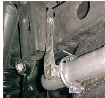
INSTALL METAL HANGER # J INTO HOLE LOCATED APPROXIMATELY 17" FROM THE REAR OF THE FRAME. USE TOP HOLE ON HANGER. INSTALL DRIVER SIDE OVERAXLE TAILPIPE # C INTO THE MUFFLER 1-1/2"-2".
