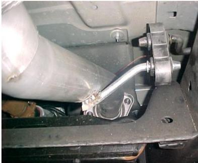
BOLT HEADPIPE # A ONTO YOUR EXISTING STOCK FRONT PIPE RE-USING FACTORY BOLTS. INSERT WELDED HANGER INTO RUBBER GROMMET.
