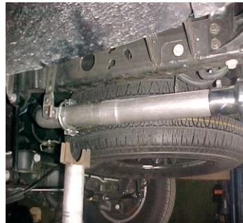
NEXT, INSTALL THE EXIT PIPES #E AND #F USING CLAMPS #H TO SECURE TO THE TAILPIPES. DO NOT TIGHTEN.
