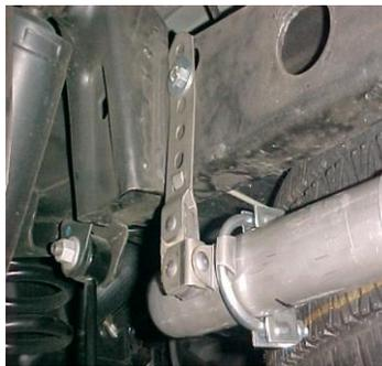
INSTALL METAL HANGER #J INTO HOLE LOCATED APPROXIMATELY 17" FROM THE REAR OF THE FRAME. USE TOP HOLE ON HANGER. INSTALL DRIVER SIDE OVERAXLE TAILPIPE # C INTO THE MUFFLER 1-1/2"-2" USING CLAMP#H. TO ATTACH PIPE TO HANGER #J USE CLAMP #H TO HOLD PIPE. DO NOT TIGHTEN.
