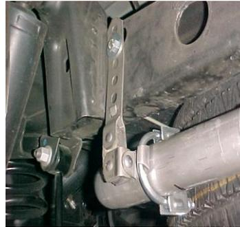
INSTALL METAL HANGER # J INTO HOLE LOCATED APPROXIMATELY 23" FROM THE REAR OF THE FRAME. USE TOP HOLE ON HANGER. INSTALL DRIVER SIDE OVERAXLE TAILPIPE # C INTO THE MUFFLER 1-1/2"-2". USE CLAMP #I TO SECURE PIPE TO MUFFLER. DO NOT TIGHTEN.
