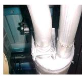
Next, install rear muffler hanger #H onto drivers side muffler outlet insert hanger into rubber grommet. Do not tighten.
