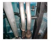
Install driverside headpipe #B. Then install headpipe #A and then Insert welded hanger into rubber grommet Secure both pipes with clamp #G. Do not tighten.
