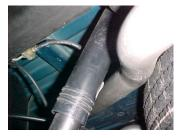
Install driverside overaxle tailpipe #E into muffler 1 ½" to 2". Long end of pipe goes into the muffler. Support end of tailpipe with stand, and attach with hanger # H.
