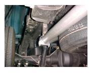
Install tailpipe hangers #J onto end of tailpipes using clamp #I. There will be about a 2" hole above the end of both tailpipes on the frame to bolt the hangers. Do not tighten.
