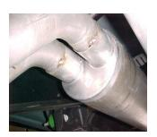
Install muffler # C onto head pipes 1-1/2" to 2" with the louvers facing towards the converter. The outlets of the muffler will be on top. Use a jack stand to support the muffler. Use clamps #G to the secure the muffler to the head pipes. Do not tighten
