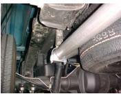
tailpipes. These clamps also attach to the metal hangers. You will need to rotate in order to adjust for clamping.
