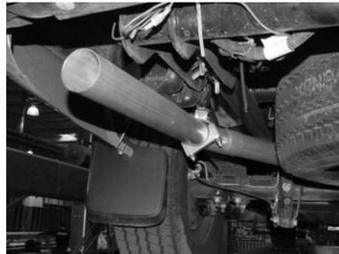
INSTALL DRIVER SIDE TAILPIPE #D INTO MUFFLER AT LEAST 1 1/2" TO 2". THIS PIPE WILL ROUTE OVER THE AXLE AND BETWEEN THE SHOCK AND SPARE TIRE. USE CLAMP #G TO SECURE PIPE TO MUFFLER. DO NOT TIGHTEN. INSERT WELDED HANGER INTO RUBBER GROMMET.
