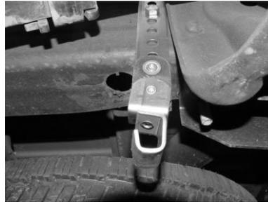
INSTALL METAL HANGERS #H INTO HOLES LOCATED APPROX. 16" FROM THE REAR OF THE FRAME. METAL HANGERS ARE MOUNTED ON THE OUTSIDE OF FRAME. USE HARDWARE KIT # I. THE BOLT AND WASHER WILL GO INTO THE 3<sup>RD</sup> HOLE FROM THE TOP OF THE HANGER.
