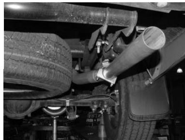
INSTALL EXIT PIPES #E ONTO TAILPIPES. CUT TO YOUR PREFERRED LENGTH USE CLAMPS #G TO SECURE EXIT PIPES TO TAILPIPES. THESE CLAMPS ALSO ATTACH TO METAL HANGERS #H. THESE METAL HANGERS NEED TO BE ROTATED IN ORDER TO ADJUST FOR CLAMPING. NOW YOU CAN TIGHTEN ALL CLAMPS, NUTS, AND BOLTS. STARTING FROM THE FRONT WORKING BACK. USE ZIP TIES TO TIE AWAY BRAKE LINES. IF YOU WOULD LIKE YOUR EXIT PIPES TO EXIT BEHIND THE REAR WHEELS ROTATE THEM TO DO SO. INSTALL STAINLESS TIPS.
