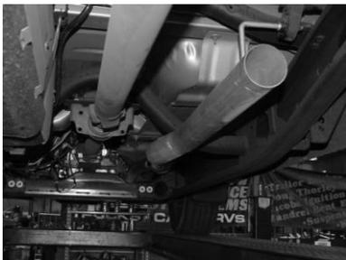
INSTALL PASSENGER SIDE TAILPIPE #C INTO MUFFLER AT LEAST 1 1/2" TO 2". USE CLAMP #G TO SECURE PIPE TO MUFFLER. DO NOT TIGHTEN. THE TAILPIPES WILL BOTH LEAN TOWARDS THE DRIVER SIDE FOR CLEARANCE.
