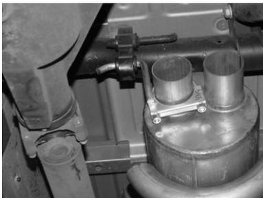
INSTALL MUFFLER #B ONTO HEADPIPE AT LEAST 1 1/2" TO 2". USE CLAMP #F TO SECURE MUFFLER TO HEADPIPE. DO NOT TIGHTEN. USE A JACK STAND TO SUPPORT THE MUFFLER. OUTLETS SHOULD BE AT THE TOP.
