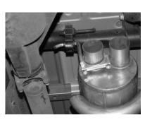
INSTALL MUFFLER #B ONTO HEADPIPE AT LEAST 1½" TO 2". USE CLAMP #F TO SECURE MUFFLER TO HEADPIPE. DO NOT TIGHTEN. USE A JACK STAND TO SUPPORT THE MUFFLER. OUTLETS SHOULD BE AT THE TOP. INSTALL HANGER #I ONTO DRIVERSIDE MUFFLER OUTLET AND INSERT WELDED HANGER INTO GROMMET. DO NOT TIGHTEN.
