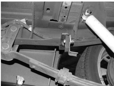
INSTALL HANGER # G ON THE PASSENGER TAILPIPE AND HANGER # H ON DRIVERSIDE TAILPIPE. MEASURE 19" FROM REAR OF FRAME AND BOLT INTO THE EXISTING ROUND HOLES (ABOUT 7/8") LOCATED ON THE FRAME ON BOTH SIDES OF THE VEHICLE.
