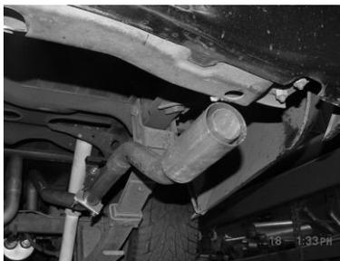
INSTALL EXIT PIPES # F ONTO OVERAXLE TAILPIPES USING CLAMP # J. ADJUST FOR YOUR PREFERENCE. NEXT ROTATE PIPES FOR BEST CLEARANCE AND ALIGN TO FRAME RAIL. TIGHTEN ALL CLAMPS AND BOLTS STARTING FROM THE HEADPIPE AND WORK BACK. INSTALL STAINLESS STEEL TIPS.
