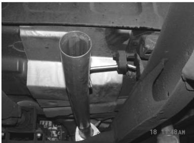
INSTALL HEADPIPE # A USING BOLT KIT # L AND # N GASKET. INSERT WELDED HANGER INTO RUBBER GROMMET AND ATTACH TO STOCK FLANGE. DO NOT TIGHTEN.
