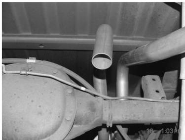
INSTALL DRIVERS SIDE FRONT TAILPIPE # D INTO MUFFLER 1-1/2" TO 2". USE CLAMP # J AND ATTACH IT TO THE MUFFLER. DO NOT TIGHTEN.
