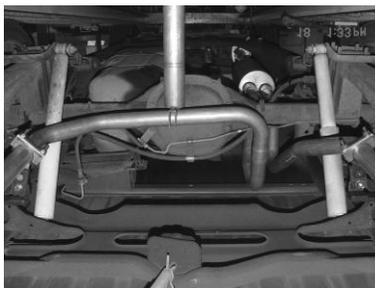
INSTALL DRIVERS SIDE OVERAXLE PIPE # E ONTO FRONT TAILPIPE USING CLAMP #J. USE CLAMP # J TO HOLD TAILPIPE UP TO REAR HANGER # H. DO NOT TIGHTEN.
