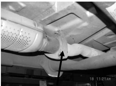
UNBOLT STOCK HEADPIPE AT THE 3 BOLT FLANGE DIRECTLY BEHIND THE CATALYTIC CONVERTER.
