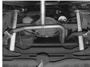
INSTALL DRIVERS SIDE OVERAXLE PIPE # E ONTO FRONT TAILPIPE USING CLAMP #I. USE CLAMP # I TO HOLD TAILPIPE UP TO REAR HANGER # G. DO NOT TIGHTEN.
