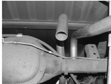
INSTALL DRIVERS SIDE FRONT TAILPIPE # D INTO MUFFLER 1-1/2" TO 2". USE CLAMP # I AND ATTACH IT TO THE MUFFLER. DO NOT TIGHTEN.
