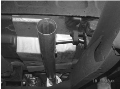
INSTALL HEADPIPE # A USING BOLT KIT # N AND # K GASKET. AND ATTACH IT TO THE STOCK FLANGE. DO NOT TIGHTEN.
