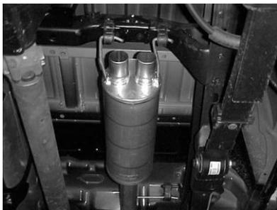
INSTALL MUFFLER #B ONTO HEADPIPE 1-1/2" TO 2" USING CLAMP #J. INSERT WELDED HANGERS INTO RUBBER GROMMET. MAKE SURE OUTLETS ARE LEVEL. USE A JACKSTAND TO SUPPORT MUFFLER. ATTACH HEADPIPE HANGER #K. DO NOT TIGHTEN.
