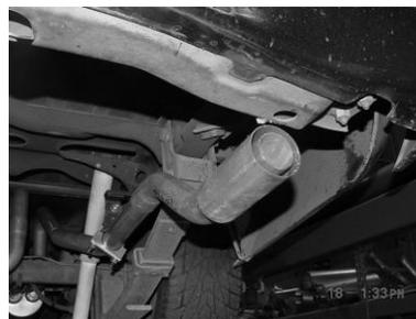
INSTALL EXIT PIPES # H ONTO OVERAXLE TAILPIPES USING CLAMP # I. ADJUST FOR YOUR PREFERENCE. NEXT ROTATE PIPES FOR BEST CLEARANCE AND ALIGN TO FRAME RAIL. TIGHTEN ALL CLAMPS AND BOLTS STARTING FROM THE HEADPIPE AND WORK BACK. INSTALL STAINLESS STEEL TIPS.
