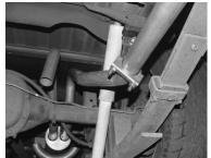
INSTALL PASSENGER SIDE TAILPIPE # C INTO THE MUFFLER 1-1/2" TO 2". ATTACH IT TO THE MUFFLER USING CLAMP # I. USE CLAMP # I TO HOLD TAILPIPE TO HANGER # F. DO NOT TIGHTEN
