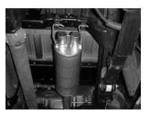
INSTALL MUFFLER #B ONTO HEADPIPE 1-1/2" TO 2" USING CLAMP #J. INSERT WELDED HANGERS INTO RUBBER GROMMET. MAKE SURE OUTLETS ARE LEVEL. USE A JACKSTAND TO SUPPORT MUFFLER. DO NOT TIGHTEN.
