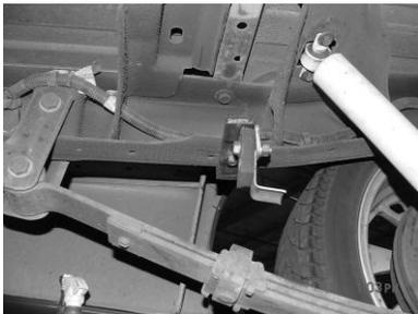
INSTALL HANGER # F ON THE PASSENGER TAILPIPE AND HANGER # G ON DRIVERSIDE TAILPIPE. MEASURE 19" FROM REAR OF FRAME AND BOLT INTO THE EXISTING ROUND HOLES (ABOUT 7/8") LOCATED ON THE FRAME ON BOTH SIDES
