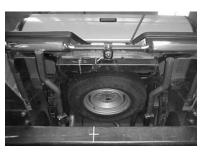
Slip the over axle tailpipes #C, #D into the outlets of the muffler no more then 1- 1/2" to 2" and attach clamp #G to passenger side and clamp hanger #I to driver side tailpipe. The driver side tailpipe will be routed over the differential between the frame and the shock. It will require some rotating of the pipe and possibly an extra person to help align the pipes when tightening the clamps. Attach hanger #H to tailpipes and attach with clamp #G.
