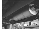
Install the muffler onto the head pipe no more then 1 1/2" to 2". Use a jack stand to support the muffler. Make sure muffler is sitting level with the vehicle and that the muffler outlets are positioned level. Level outlets across at 12'oclock position.
