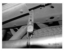
REMOVE STOCK REAR HANGER FROM FRAME ON PASSENGER SIDE.
