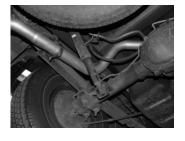
INSTALL DRIVERSIDE TAILPIPE #D INTO MUFFLER 1-1/2" TO 2". THIS PIPE GOES BETWEEN THE SHOCK & FRAME. SLIDE CLAMP #G OVER PIPE AND CONNECT IT TO THE HANGER #H. THIS WILL HOLD UP THE TAILPIPE. ATTACH TAILPIPE TO MUFFLER OULET USING CLAMP #I.
