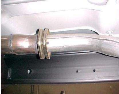
TO REMOVE STOCK EXHAUST UN-BOLT IT FROM THE 2-BOLT FLANGE LOCATED JUST BEHIND THE Y-PIPE. **DO NOT DAMAGE FACTORY HARDWARE, YOU WILL RE-USE IT.** NOW CUT OFF YOUR STOCK TAILPIPE JUST BEHIND THE MUFFLER AND REMOVE. LEAVE ALL RUBBER GROMMETS ON THE HANGER. USE WD-40 TO AID IN REMOVAL OF EXHAUST AND HANGERS.
