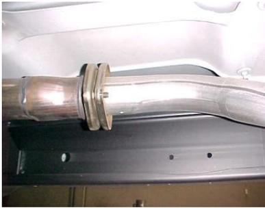
LAY OUT THE GIBSON EXHAUST ON THE FLOOR SO IT LOOKS LIKE THE DRAWING AND COMPARE PART #'S WITH MANUAL. TO REMOVE YOUR STOCK EXHAUST, REMOVE IT FROM THE STOCK 2-BOLT FLANGE LOCATED JUST BEHIND THE CONVERTER, LEAVING ALL RUBBER GROMMETS IN PLACE. USE WD-40 TO AID YOU IN REMOVAL OF EXHAUST AND HANGERS. **DO NOT THROW AWAY FACTORY HARDWARE. YOU WILL RE-USE IT.**
