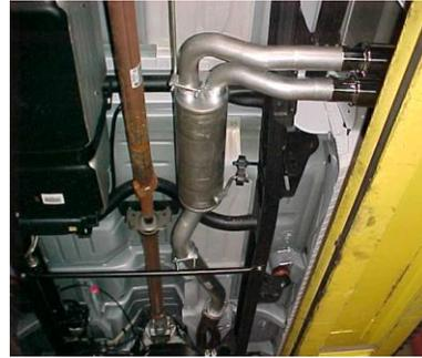
INSTALL MUFFLER ASSEMBLY #B ONTO HEADPIPE #A. SLIDE WELDED HANGERS INTO RUBBER GROMMETS. USE CLAMP #C TO SECURE MUFFLER ASSEMBLY TO HEADPIPE. DO NOT
