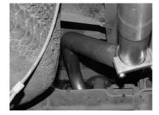
INSTALL PASSENGER SIDE TAILPIPE #C INTO MUFFLER 1-1/2" TO 2" USING CLAMP #I THEN ATTACH WITH CLAMP #H AND ATTACH TO MUFFLER. ATTACH HANGERS #I TO BOTH TAILPIPES. ATTACH WITH CLAMP #H. DO NOT TIGHTEN.
