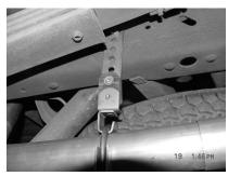
INLET TOWARDS CONVERTER USING CLAMP #G TO SECURE MUFFLER TO HEADPIPE. USE A JACKSTAND TO SUPPORT THE MUFFLER. DO NOT TIGHTEN. BEMOVE STOCK BEAB
