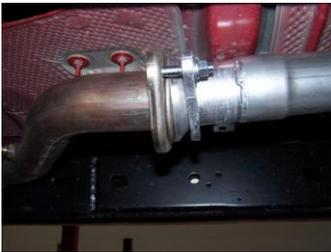
3. Install headpipe #A onto your existing stock 2-bolt flange. Use bolt kit #J to secure. Use jack stand to support converter. Install front muffler hanger #F. Insert hanger into rubber grommet. Do not tighten.
