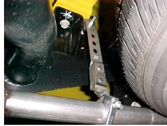
5. Install the driver side rear tailpipe hanger #G and clamp #H. It should be installed just in front of the rear bed mount on the driver side.
