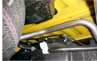
6. Install driver side tailpipe #C into muffler 1.5-2". Rotate until it touches the rear mount, use clamp #H to secure tailpipe to muffler. Do not tighten.
