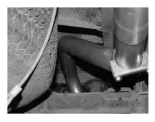
INSTALL EXIT PIPES #E ONTO TAILPIPES. ROLL EXIT PIPES UNTIL YOU HAVE THE CORRECT ANGLE. USE CLAMP #H TO SECURE THESE TO THE TAILPIPES. DO NOT TIGHTEN. CUT EXIT PIPE TO PROPER LENGTH.
