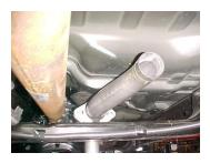
Lay out the exhaust on the floor so it looks like the drawing and compare parts with manual. To remove your stock exhaust Remove it from the 2-bolt flange located in front of the muffler. Then cut off your tailpipe. Leave all rubber grommets in place. Use WD-40 to aid in removal of exhaust and hangers.
