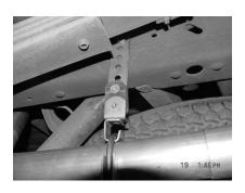
REMOVE STOCK REAR HANGER FROM FRAME ON PASSENGER SIDE. INSTALL 10" METAL HANGER #I. USE THE FIFTH HOLE FROM THE BOTTOM. INSTALL IT IN THE TOP FACTORY HOLE WHERE THE STOCK HANGER WAS IN. IT IS LOCATED APPROX. 20" FROM REAR OF FRAME 3/8" HOLE.REPEAT FOR THE DRIVERSIDE.
