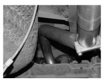
INSTALL EXIT PIPES #E C NTO TAILPIPES. ROLL EXIT PIPES UNTIL YOU HAVE THE CORRECT ANGLE. USE CLAMP #H TO SECURE THESE TO THE TAILPIPE. DO NOT TIGHTEN. CUT EXIT PIPE TO PROPER LENGTH.
