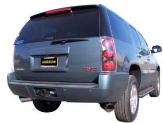
9. Install stainless steel tip. Clamp down. When you have everything in place, firmly tighten all bolts and clamps down securely. Use stainless steel or aluminum cleaner to prevent tip from discoloration. Inspect all fasteners after 25-50 miles of operation and re-tighten as necessary.
