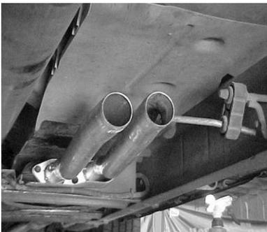
Bolt head pipe #A to the stock head pipe flange behind the converter reusing stock bolts and supplied gasket. Use a Hi-Temperature O2 sensor safe silicone on the gasket for a good seal. Insert welded hanger side into rubber grommet. Re-install O2 sensor into head pipe. Apply a small amount of anti-seize on the threads. Do not tighten.
