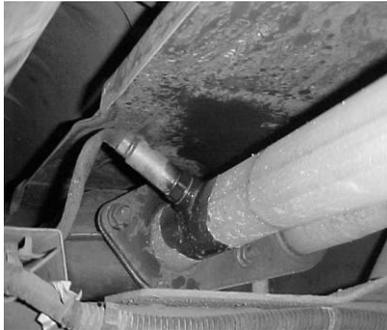
Remove O2 sensor from stock head pipe and remove stock flange gasket. You will reuse the stock bolts.
