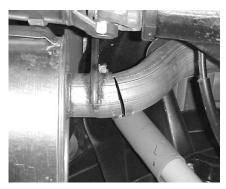
LAYOUT THE GIBSON EXHAUST AS SHOWN ON YOUR MANUAL. COMPARE THE PIPE NUMBERS TO THE MANUAL NUMBERS, MAKE SURE THEY ALL MATCH. THEN, CUT THE STOCK TAILPIPE OFF JUST AFTER THE MUFFLER FOR EASY REMOVAL.
