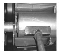
INSTALL MUFFLER # B ONTO HEADPIPE #A 12" TO 2". THE INLET WILL BE AT **APPROXIMATELY** 6 O'CLOCK, CONNECT THE MUFFLER TO HEADPIPE#A USING CLAMP#F. INSERT WELDED HANGER INTO RUBBER GROMMET.
