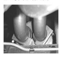
INSTALL TAILPIPES # C & D USE CLAMP#G ON THE PASSENGER SIDE AND HANGER #I ON THE DRIVER SIDE, INSERT WELDED HANGER INTO RUBBER GROMMET. USE BOLT KIT#H TO CONNECT BOTH THE TAILPIPES TOGETHER.
