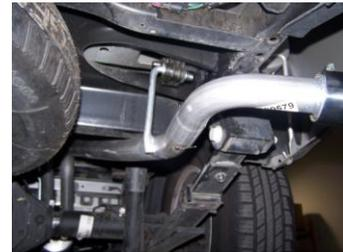
Install passenger side tailpipe #D into muffler 1 1/2" to 2". Insert welded hanger into rubber grommet. Use clamp # H to secure. Do not tighten.
