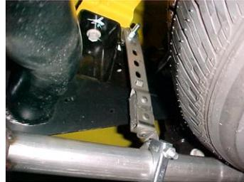
Next, install driverside rear tailpipe #C with hanger # G, Attach with clamp #H, it will be installed just in front of the rear bed mount on the drivers side.
