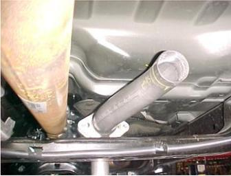
Install head pipe # A on to your existing stock 2-bolt flange use bolt kit #J to secure. Leave loose until the whole system is installed.
