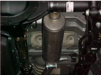
Install muffler #B onto head pipe #A 1-1/2" to 2" with the louvers facing towards the converter. Use a jack stand to support the muffler. Outlet of muffler will be level.
