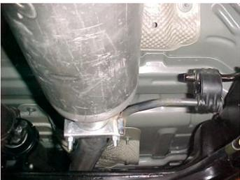
Next install front muffler hanger #F onto muffler. Insert hanger into rubber grommets. Do not tighten.
