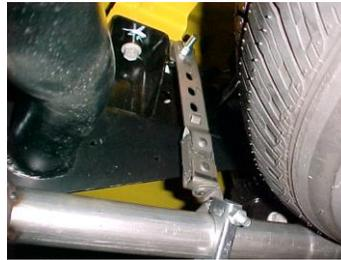
6. Next, install the driver side rear tailpipe hanger (#G) and clamp (#H). It will be installed just in front of the rear bed mount on the driver side.
