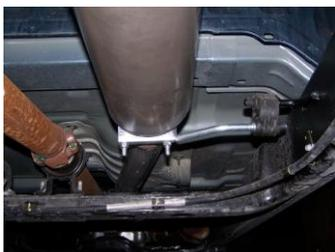
5. Next, install front muffler hanger #F onto muffler. Insert hanger into rubber grommets. Do not tighten.
