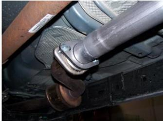
3. Install headpipe (#A) onto your existing stock 2-bolt flange. Use bolt kit (#J) to secure. Leave loose until the whole system is installed.
