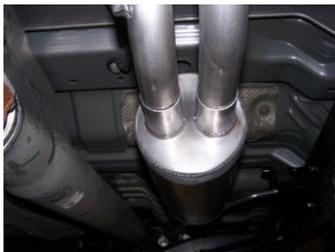
4. Install muffler (#B) onto headpipe (#A) 1.5-2" with louvers facing towards the converter. Use a jack stand to support the muffler. Outlet of muffler will be level.
