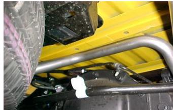
7. Install driver side tailpipe (#C) into muffler 1.5-2". Rotate until it touches the rear mount, use clamp (#H) to secure tailpipe to muffler. Do not tighten.
