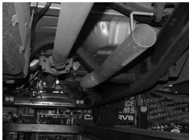
INSTALL THE PASSENGER SIDE TAILPIPE #C INTO MUFFLER AT LEAST 1 1/2" TO 2". USE CLAMP (#G) TO SECURE PIPE TO MUFFLER. DO NOT TIGHTEN. THE TAILPIPES WILL BOTH LEAN TOWARDS THE DRIVER SIDE LOOKING FROM THE REAR OF THE VEHICLE - THIS TAILPIPE IS AT APPX. 11 O'CLOCK.
