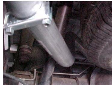
INSTALL THE DRIVER SIDE TAILPIPE #D INTO MUFFLER AT LEAST 1 1/2" TO 2". THIS PIPE WILL THEN ROUTE OVER THE AXLE AND BETWEEN THE SHOCK AND TIRE. ATTACH CLAMP (#I) TO SECURE TAILPIPE TO MUFFLER. DO NOT TIGHTEN. LOOKING FROM THE REAR OF THE VEHICLE - THIS TAILPIPE IS AT APPX. 11
