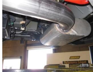
4. Once you have entire system hanging loose re install the factory frame support bracket. Install the forward bolt loosely and used the supplied spacers and bolts for the rear 6 bolts. Tighten down all the bolts.
