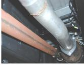
3. Disengage the welded hangers from the OEM rubber grommets. Use WD-40 to aid in the process. Do not damage or remove the rubber grommets as you will re-use them. Now, cut off tailpipe and remove exhaust. You also will re-use your factory nuts.
