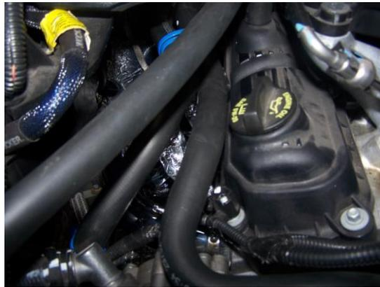
7. AFTER HEADERS ARE IN PLACE. RE-INSTALL FACTORY Y-PIPE ASSEMBLY USING SUPPLIED BOLT KIT. NOW RE-CONNECT BATTERY. CHECK FOR ALL PROPER CLEARANCES THEN START VEHICLE AND THEN CHECK FOR ANY LEAKS. AFTER WARM-UP LET VEHICLE COOL DOWN AND RETORQUE ALL FASTENERS.
