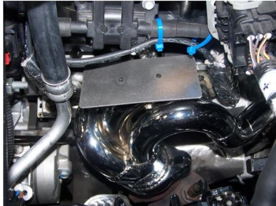
4. INSTALL THE HEAT SHIELD 5" X 8" ON THE PASSENGER SIDE # 1 CYLINDER TUBE TO PROTECT THE BATTERY BOX. THIS WILL PREVENT HEAT GOING TO COIL PACK ABOVE HEADER ASSEMBLY.
