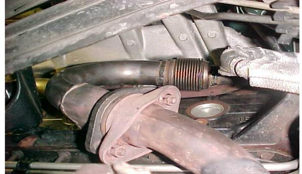
4. DISCONNECT THE O2 SENSOR PLUG FROM BRACKET NEXT TO THE OIL PAN. THEN DISCONNECT STOCK HEADPIPE FROM MANIFOLD. THEN REMOVE DRIVERSIDE MOTOR MOUNT ON ENGINE (**ONLY ON CHEROKEE MODELS. WRANGLER DO NOT**) TO HELP AID IN REMOVAL OF MANIFOLD AND INSTALLATION OF HEADER. "**NOTE: USE FLOOR JACK TO SUPPORT THE WEIGHT OF THE ENGINE ON CHEROKEE MODELS ONLY!**"
