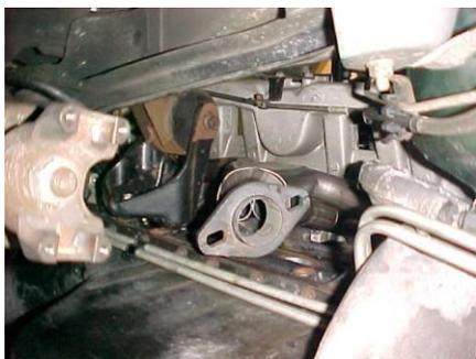
7. RE-INSTALL MOTOR MOUNT. **(ONLY ON CHEROKEE MODELS)** PLUG IN O2 SENSOR, INSTALL NEW SUPPLIED DONUT GASKET FOR HEADPIPE CONNECTION. THEN ATTACH HEADPIPE TO HEADER WITH NEW SUPPLIED EXHAUST DONUT. TORQUE HEADPIPE TO 30-35 FTS.
