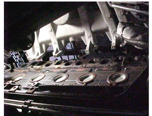
6. INSTALL GIBSON HEADER WITH SUPPLIED GASKET. AFTER HEADER IS BOLTED UP ON BOTH ENDS OF HEAD. INSTALL INTAKE MANIFOLD BACK ON, TORQUING ALL FASTENERS TO 35 - 35 FTS.
